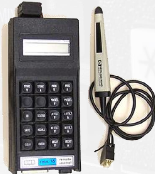
Image of an original RMX16 remote control with bar code reader
