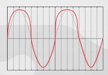
reaching the non-linear regions of the transfer curve. This is typically associated with the classic "warm," "thick," and "analog" sound.
