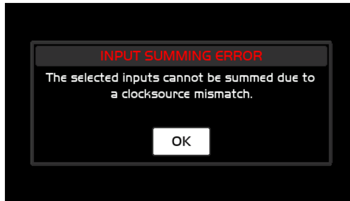
Illustration 13: Input Summing Error: clocksource mismatch
