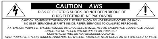
The lightning flash with arrowhead symbol within an equilateral triangle is intended to alert the user to the presence of uninsulated "dangerous voltage" within the product's enclosure, that may be of sufficient magnitude to constitute a risk of electric shock to persons.
