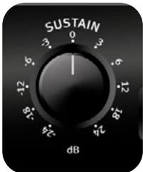
Sustain can be used to increase or attenuate the sustain phase of a signal by up to 24 dB. Positive sustain values extend the sustain. Negative Sustain values shorten the sustain.
