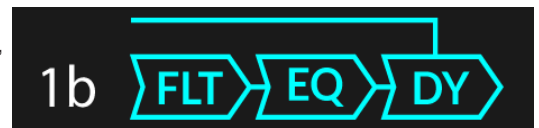
'b' equivalent - the top line going into Dynamics means that the Dynamics sidechain is set to EXTERNAL
