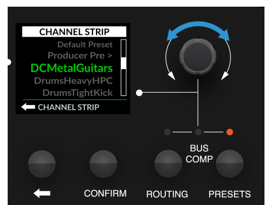
Navigate through your presets list using the secondary encoder and push to load
